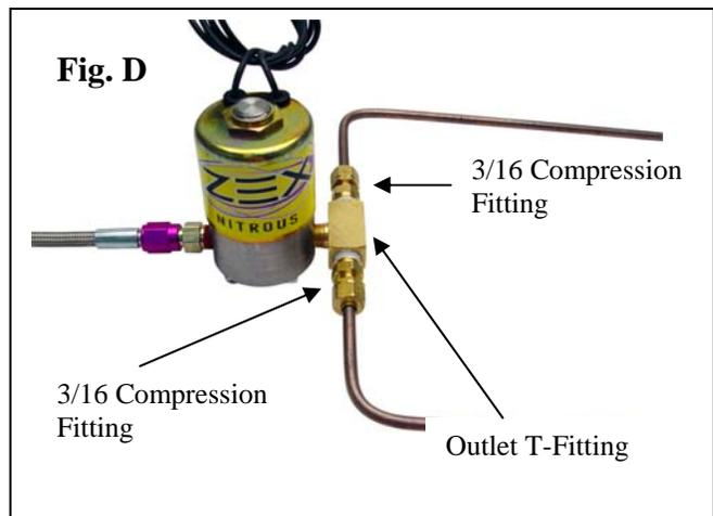
8. Bend the hard-line to your specifications and then attach and tighten them to the two outlet compression fittings (Fig. D).
