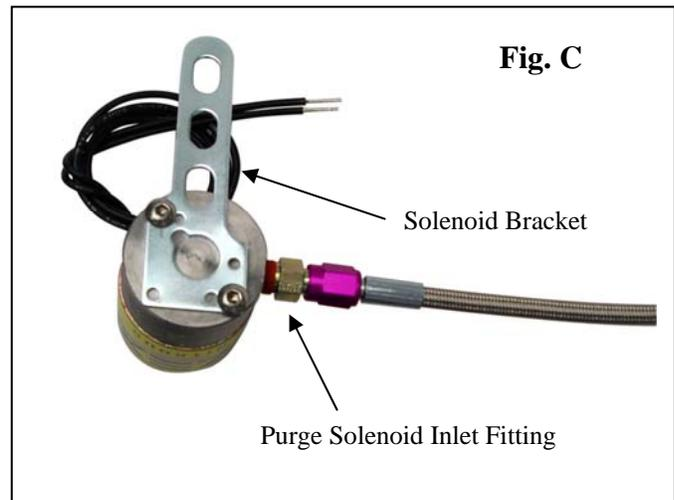
6. Find an appropriate place for the solenoid bracket, keeping in mind that you will need to place it in an area that will allow you to route the two q3w in. hard-lines to your desired nitrous discharge areas. Attach the bracket using the two large sheet metal screws included with the kit. Fasten the purge solenoid to the bracket with the two enclosed Allen head screws (Fig. C).
